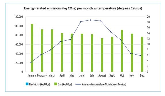
The primary axis (left) of the above graph shows the energy-related emissions for the components 'electricity' and 'gas' per month in relation to the average outdoor air temperature in the Netherlands for the same month on the secondary axis (right).
